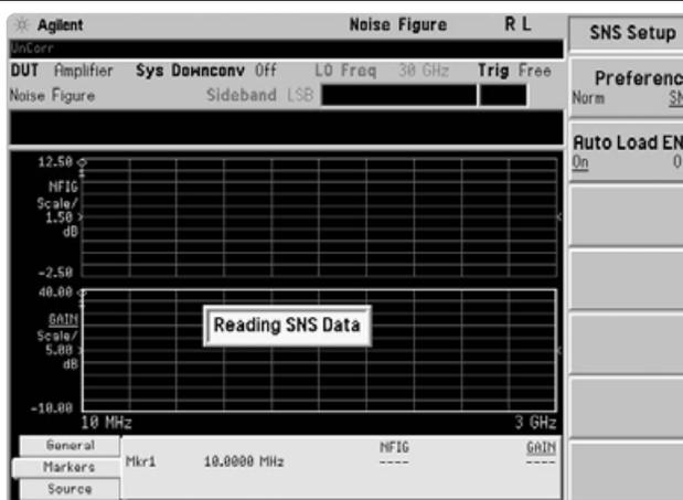
If the noise source preference was a normal 346 Series noise source, then this is the same interface that you would use to enter the ENR data. The 346 Series comes with a disk containing the noise source ENR data. Load it as follows.
